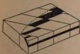
FIG. 46.—A series of parallel faults indicated by successive offsets in the course of an easily recognizable rock formation.
